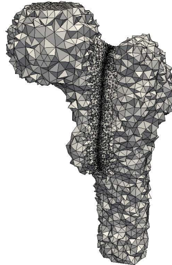
(b) Immersogeometric tetrahedral mesh of finite cells that locally refine the fracture region.
